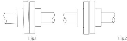
When correcting any defects in coupling alignment, the errors of angularity should be checked and rectified before correcting any errors of eccentricity.
