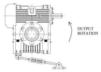
V. Attach the unit to a stable foundation using the foot bracket of the torque arm. Attempt to locate the foot bracket so that the torque arm will be at approximately right angles to the centre line created through the driven shaft and the torque arm pivot pin (as shown on the previous page). This angle may vary up to a maximum of 30° in either direction where necessary.
